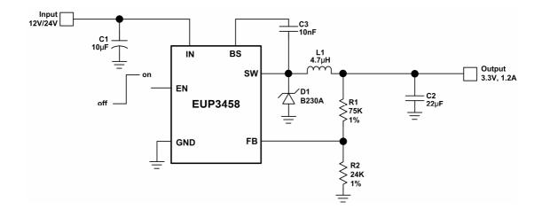
Figure 1. 12V/24V to 3.3V Application Circuit
